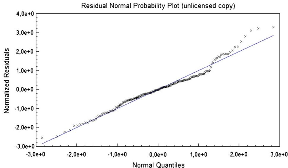
**Fig. 1.** Normal probability plot of the residuals. A normal distribution is evidenced by the points roughly lying on a straight line. The plot demonstrates adequate normality of the residuals. The discrepant high data have not been removed from the analysis.
